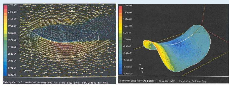
High Speed Conveying Create Vortices Shedding... ...'Rocking Chips' NOT GOOD!
